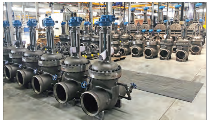
Cast steel valves for NTPC Telangana supercritical power plant manufactured and ready for shipment from our Velan Valves India location.
