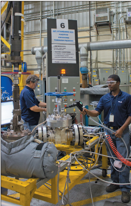
API 624 fugitive emissions qualification testing.
