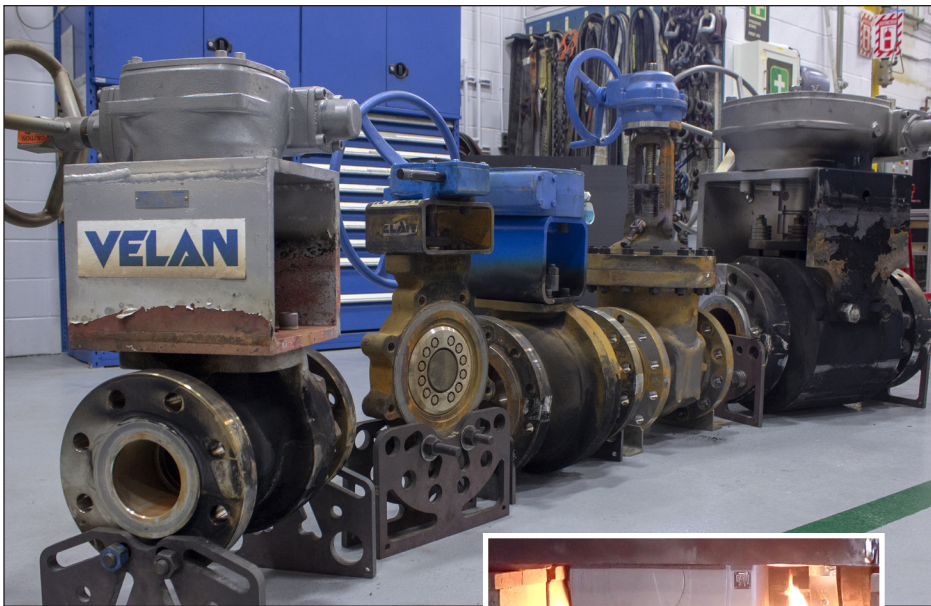
Above: Five Velan valves, including two Securaseal R-series metal-seated ball valves, fire tested to the latest API and ISO standards.
