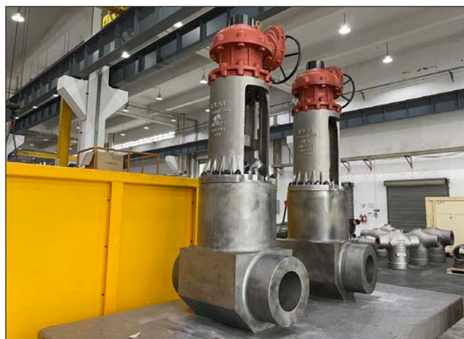
Two 24" Class 2500 gate valves in Velan Valves (Suzhou) plant to be installed in a refining and petrochemicals complex in China. The project was a team effort with collaboration between our plants in China, Korea, Italy, and Canada.
